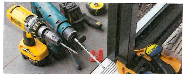
Generally, only battery-powered or 110 volt tools are permitted on site
