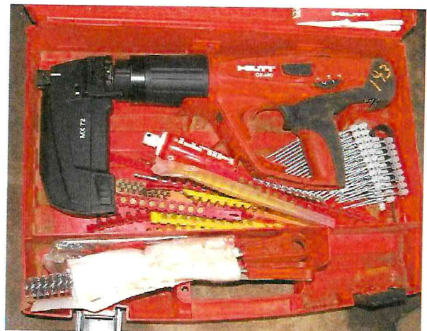
Safe storage of a cartridge tool
