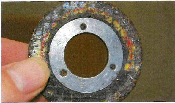
Abrasive wheel too small due to excessive use, and a snagging hazard
