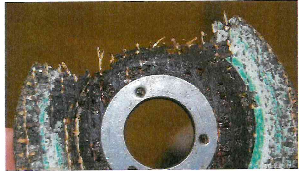
Failure caused by poor storage or age of disc
