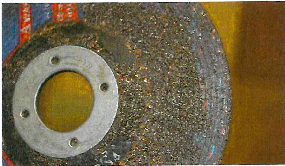
Extreme thermal damage caused by faulty machine bearings
